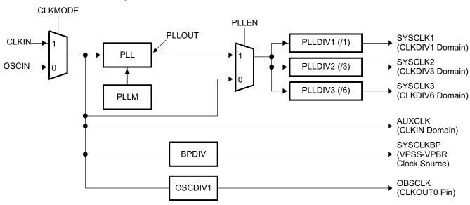
Figure 5-1. PLL1 Structure in the TMS320DM643x DMP
